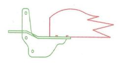
INSTALL GRILLE GUARD MOUNT WITH TOW POINT TOWARDS THE CENTERLINE OF THE VEHICLE. RE-USE FACTORY BOLTS.
