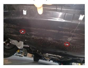
13. Remove the two 13mm bolts that are shown in the photo below. Right below the bolts that were just removed, cut a  $\frac{1}{2}$  x 1" slot to allow the lower mount to pass through.
