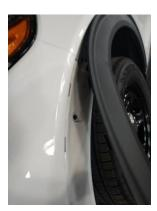
5. Pull the inner wheel liner down to access the two 10mm bolts that attach the bumper skin to the fender. Repeat for the other side.
