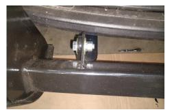
18. Separate the bumper skin and the lower splash shield to reach in and tighten the bolts on the lower mount.
