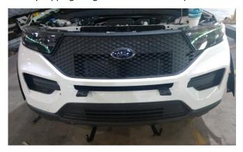
16. Set the grille guard on top of the upper mounts and start the six  $\frac{1}{2}$ " provided bolts.
