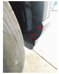
3. Remove the four 7mm bolts from the front of the inner wheel liner.
