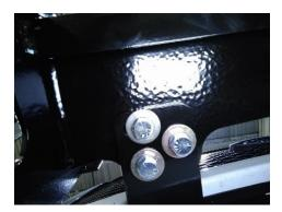
17. Attach the lower mount to the guard using the provided 1  $\frac{1}{2}$ " hardware.
