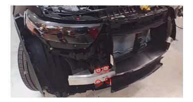
10. Start the tow lug of the aluminum bumper into the square cutout of the TS upper mount and rotate the bumper into place. Align the perimeter of the square mounting pads of the TS upper mount and the aluminum mount. Install the 3/8" hardware that is provided onto the TS mount and tighten completely.
