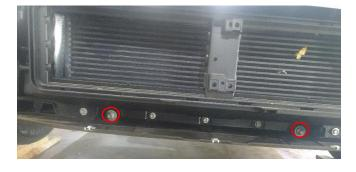
14. Install the lower mounts using the two 13mm bolts (removed in step #13) as shown and start the bolts. Do not tighten at this time. Re-install the duct work.
