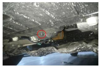
8. Pull at the edge of each wheel well to unsnap bumper skin from the fender and underneath the headlight. Reach between the bumper skin and the wheel well liner to disconnect the fog light wiring harness on the passenger side. Remove the skin.
