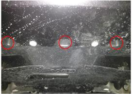
6. Remove the two 13mm bolts that hold the front of the transmission skid plate.
