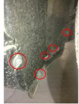
5. Remove the three 10mm bolts located at the bottom of the bumper skin.
