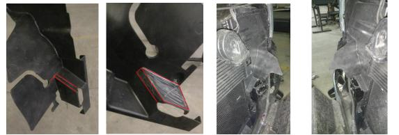
14. Install new radiator support struts attaching to the upper mount, using the provided ¼" hardware on lower end of strut.
