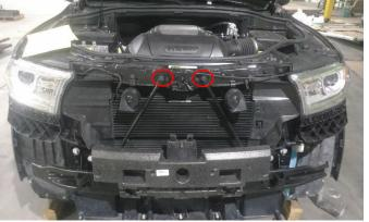
10. Remove the two 10mm bolts located on the internal bumper.
