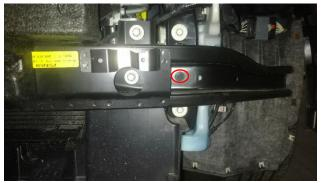
11. Remove the four 13mm bolts that attach to the internal bumper and remove.
