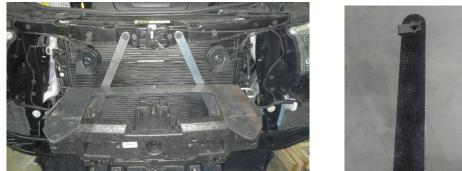
15. Trim brake duct work and rear bumper skin mount as shown in the photo. Trim duct work 4 ½" and 7 ½" (see picture).
